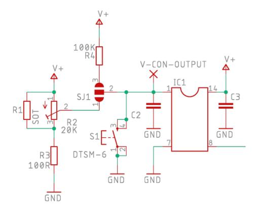
Most SPXO and TCXO products include a function to stop the output of the device by inputting a logic 1 or logic 0 to Pad 1 of the oscillator.
