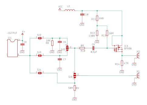
For optimum performance oscillators must have correct loading between the RF output and the input of the following device. Incorrect loading can result in increased current draw within the oscillator which can cause internal heating and thus affect the frequency stability.
