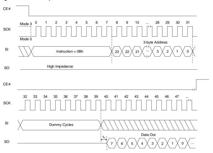
Note: Dummy cycles depends on Read Parameter setting. Detailed information in Table 6.11 Read Dummy Cycles.
