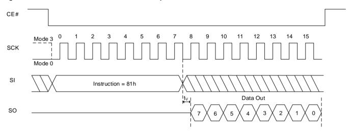
Figure 8.47 Read Extended Read Parameters Sequence In QPI Mode
