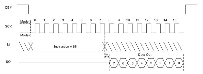
Figure 8.45 Read Read Parameters Sequence In QPI Mode
