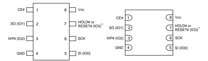
8-pin SOIC 208mil (Package: B) 8-pin SOIC 150mil (Package: N) 8-pin VVSOP 150mil (Package: V) 8-pin USON 2x3mm (Package: U) 8-pin USON 4x3mm (Package: T) 8-pin WSON 6x5mm (Package: K)
