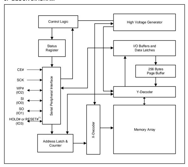
Note1: According to the P7 bit setting in Read Register, either HOLD# (P7=0) or RESET# (P7=1) pin can be selected.
