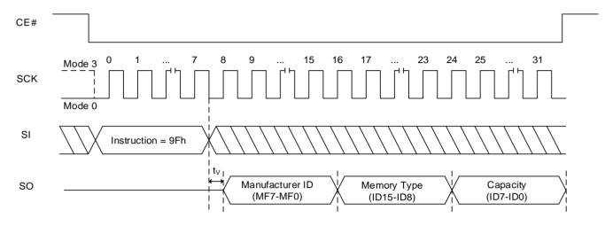
Figure 8.53 RDJDIDQ (Read JEDEC ID In QPI Mode) Sequence
