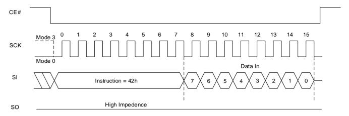
Figure 8.33 Write Function Register QPI Sequence In QPI Mode
