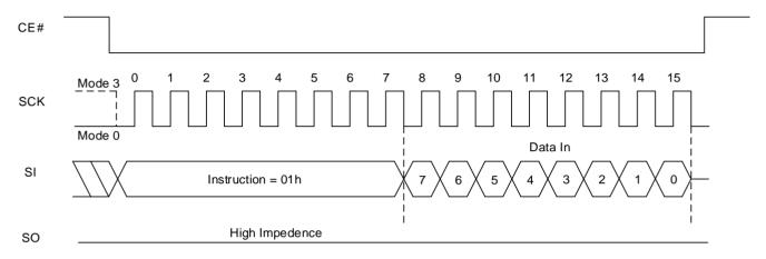
Figure 8.29 Write Status Register Sequence In QPI Mode
