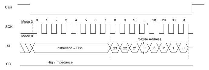
Figure 8.17 Block Erase (64K) Sequence In QPI Mode
