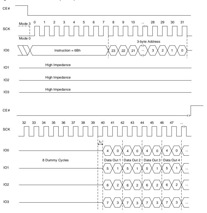
Note: Dummy cycles depends on Read Parameter setting. Detailed information in Table 6.11 Read Dummy Cycles.
