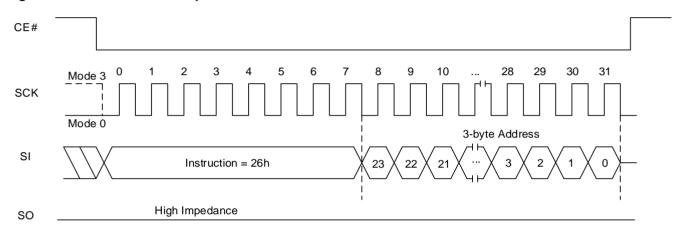
Figure 8.71 Sector Unlock QPI Sequence In QPI Mode
