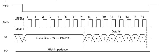
Figure 8.41 Set Read Parameters Sequence In QPI Mode
