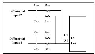
Figure 12 Summing Two Differential Inputs
