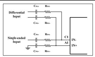
Figure 13 Summing Differential Input and Single-Ended Input Signals
