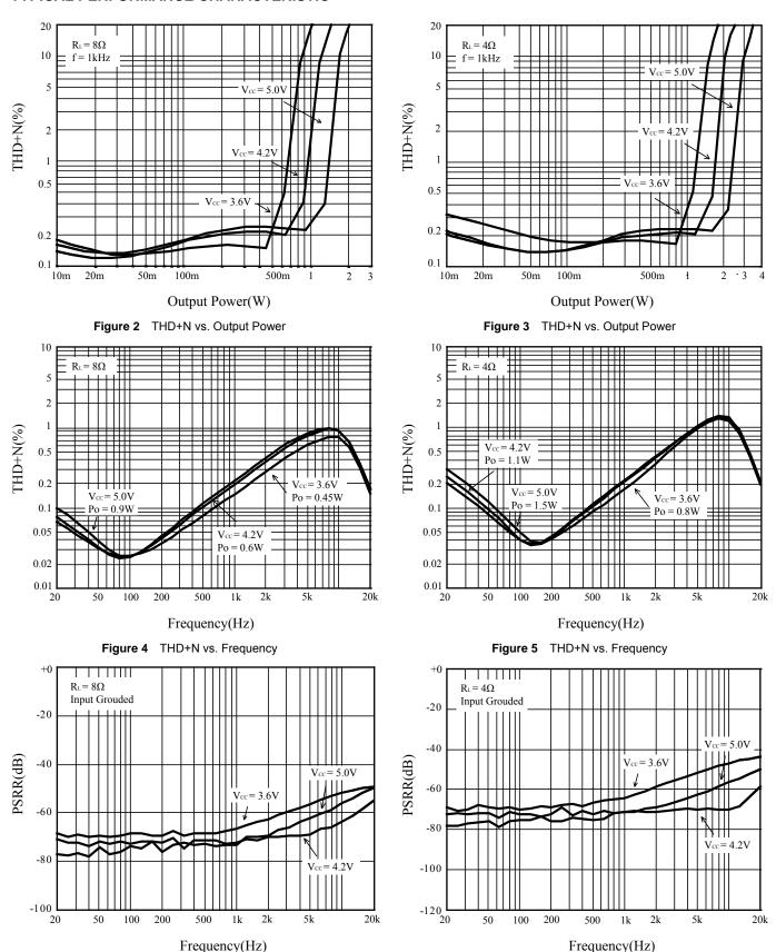
Figure 6 PSRR vs. Frequency
