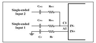
Figure 14 Summing Two Single-Ended Inputs
