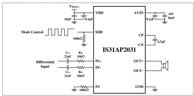
Figure 1 Typical Application Circuit (Differential Input)
