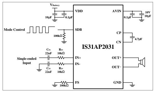
Figure 2 Typical Application Circuit (Single-ended Input)
