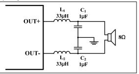
Figure 25 Typical LC Output Filter for  $8\Omega$  Speaker
