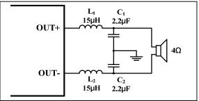
Figure 26 Typical LC Output Filter for  $4\Omega$  Speaker
