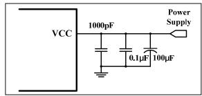
Figure 27 Recommended Power Supply Decoupling Capacitors
