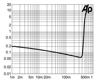
Figure 3 THD+N vs. Output Power 3V, 8Ohm, BTL at f=1kHz
