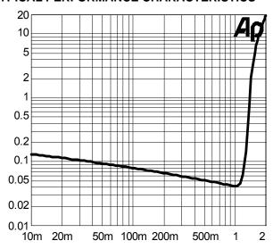
Figure 2 THD+N vs. Output Power 5V, 8Ohm, BTL at f=1kHz
