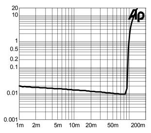
Figure 4 THD+N vs. Output Power SE mode, 5V, 32Ohm, f=1kHz
