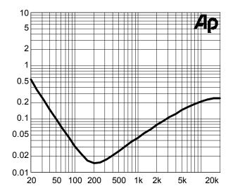
Figure 8 THD+N vs. Frequency BTL mode, 5V, 8Ohm, Po=800mW
