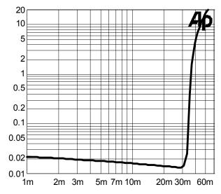
Figure 5 THD+N vs. Output Power SE mode, 3V, 32Ohm, f=1kHz
