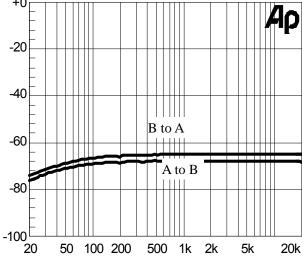
Figure 29 Crosstalk SE mode, 3V, 32Ohm, Po=30mW
