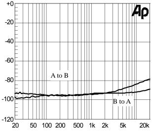
Figure 27 Crosstalk BTL mode, 3V, 8Ohm, Po=0.3W
