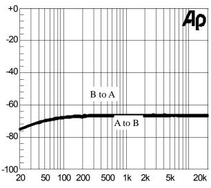
Figure 28 Crosstalk SE mode, 5V, 32Ohm, Po=80mW
