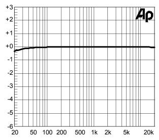
Figure 23 Frequency Response BTL mode, 3V, 8Ohm
