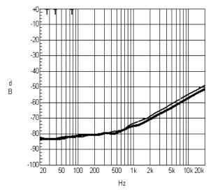
Figure 14 PSRR vs. Freq BTL mode, 5V, 8Ohm, 200mVpp Input terminated
