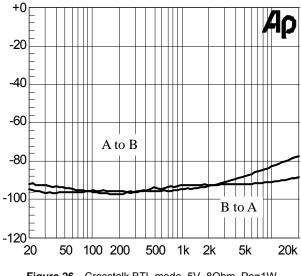
Figure 26 Crosstalk BTL mode, 5V, 8Ohm, Po=1W
