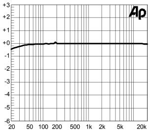
Figure 22 Frequency Response BTL mode, 5V, 8Ohm
