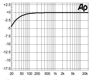
**Figure 24** Frequency Response SE mode, 5V, 32Ohm, C5/C6=220uF
