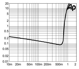
Figure 7 THD+N vs. Output Power BTL mode, 3V, 4Ohm, f=1kHz
