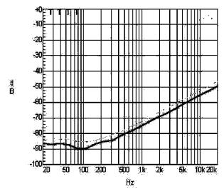
Figure 17 PSRR vs. Freq BTL mode, 3V, 8Ohm, 200mVpp Input unterminated
