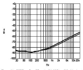
Figure 21 PSRR vs. Freq SE mode, 3V, 32Ohm, 200mVpp Input unterminated
