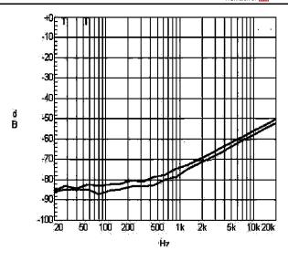
Figure 15 PSRR vs. Freq BTL mode, 3V, 8Ohm, 200mVpp Input terminated
