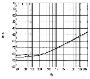
Figure 16 PSRR vs. Freq BTL mode, 5V, 8Ohm, 200mVpp Input unterminated
