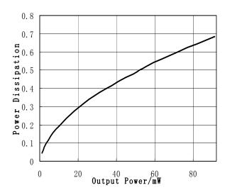
Figure 31 Power Dissipation vs. Output Power SE mode, 5V, f=1 kHz, RL=32Ohm
