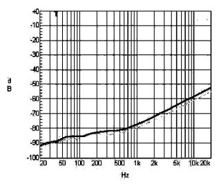
Figure 20 PSRR vs. Freq SE mode, 5V, 32Ohm, 200mVpp Input unterminated
