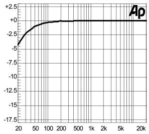
**Figure 25** Frequency Response SE mode, 3V, 32Ohm, C5/C6=220uF
