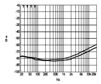
Figure 18 PSRR vs. Freq SE mode, 5V, 32Ohm, 200mVpp Input terminated
