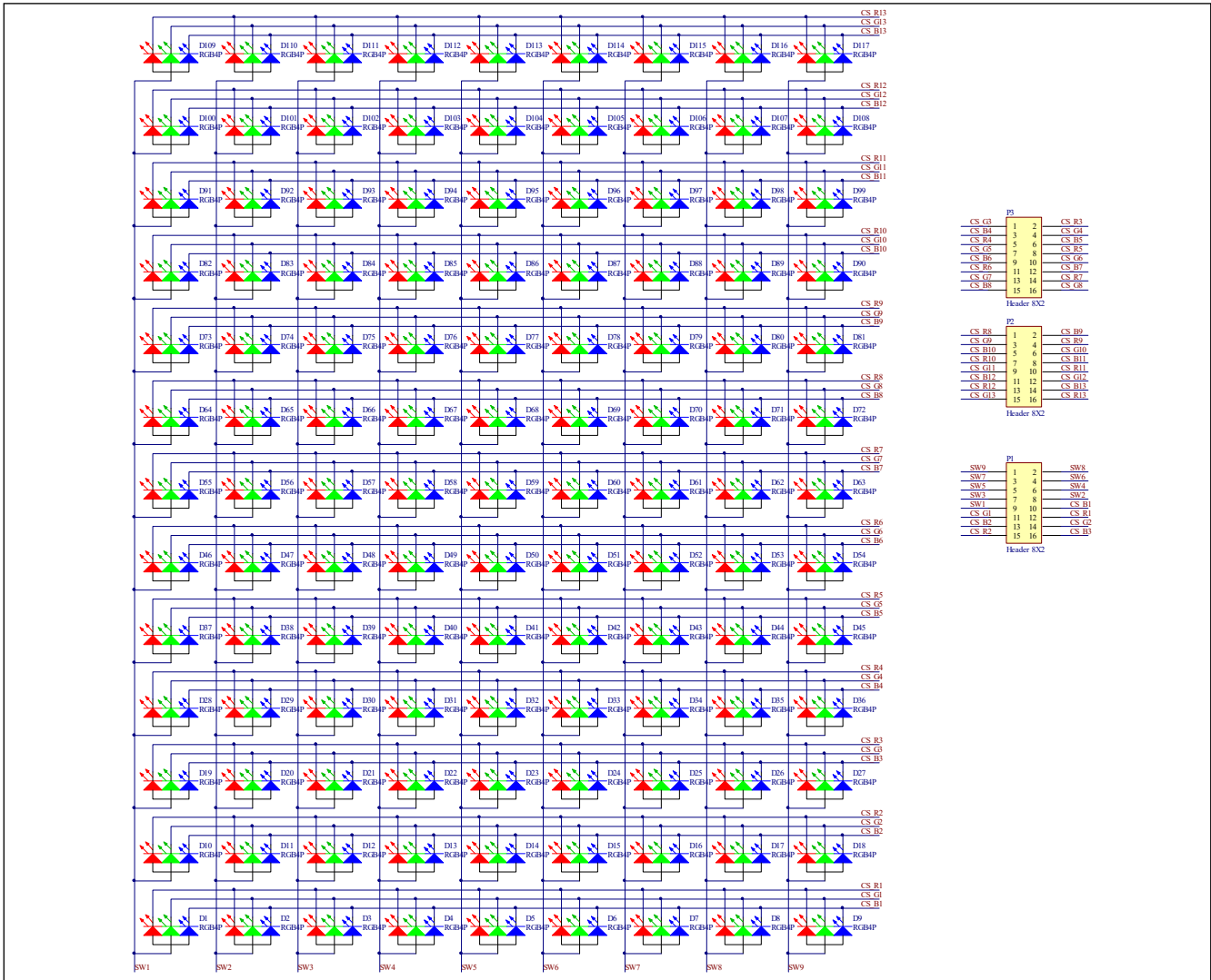
Figure 4: FxLED_9x13_ARRAY Application Schematic
