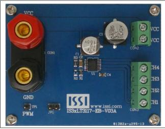
Figure 1: Photo of IS31LT3117 Evaluation Board
