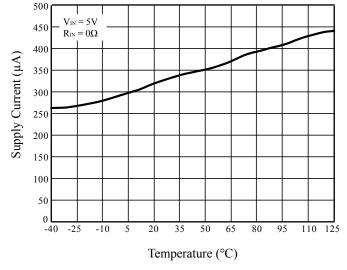
Figure 12 Temperature vs. Supply Current
