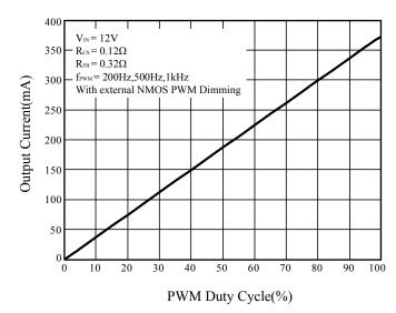
Figure 11 PWM Duty Cycle vs. Output Current
