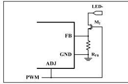
Figure 17 External PWM Dimming
