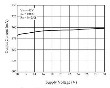
Figure 2 Supply Voltage vs. Output Current
