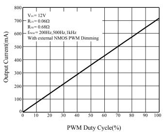
Figure 10 PWM Duty Cycle vs. Output Current
