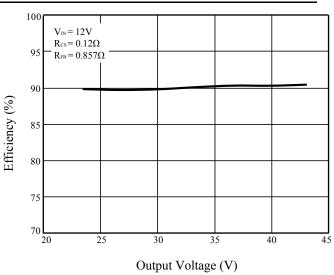
Figure 9 Output Voltage vs. Efficiency
