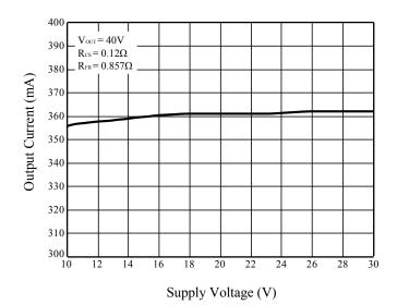
Figure 3 Supply Voltage vs. Output Current
