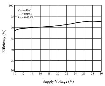
Figure 4 Supply Voltage vs. Efficiency
