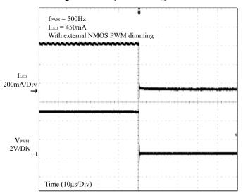
$\textbf{Figure 16} \quad \text{Output Current vs. } V_{\text{PWM}} \text{ on Falling Time}$
