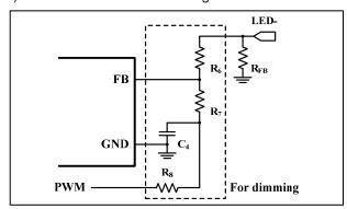
Figure 18 RC PWM Dimming
