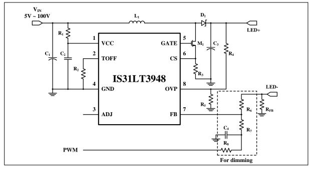
Figure 21 RC Filter PWM Dimming
