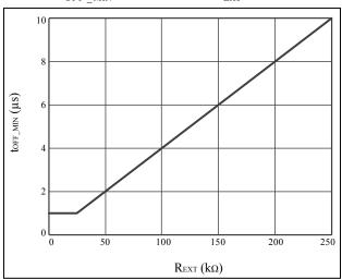
Figure 19 R<sub>EXT</sub> vs. t<sub>OFF\_MIN</sub>
