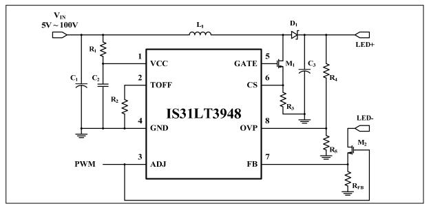
Figure 20 External NMOS PWM Dimming
