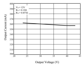
Figure 7 Output Voltage vs. Output Current
