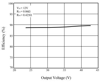
Figure 8 Output Voltage vs. Efficiency
