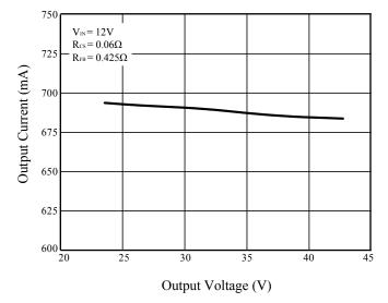
Figure 6 Output Voltage vs. Output Current
