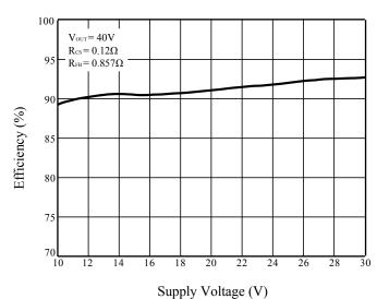
Figure 5 Supply Voltage vs. Efficiency
