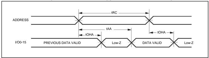
READ CYCLE NO.  $2^{(1,3)}$  ( $\overline{CS1}$ , CS2,  $\overline{OE}$ , AND  $\overline{UB}$  &  $\overline{LB}$  CONTROLLED)
