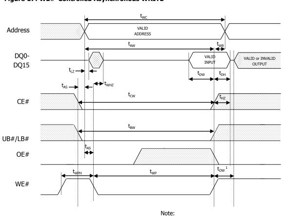
Figure 17: WE#-Controlled Asynchronous WRITE
