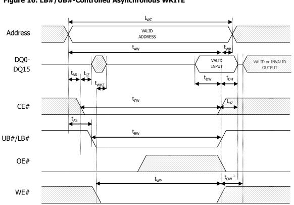
Figure 16: LB#/UB#-Controlled Asynchronous WRITE
