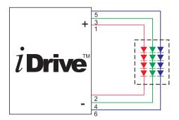
These typical are wiring configurations many other combinations can be used including white LED systems.
