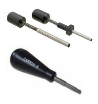
Contacts can readily be removed from the housings using an extraction tool. The tool is placed over the contact and the sleeve rotated slightly as it is pushed home to release the spring. Light pressure on the knob then ejects the contact from the rear of the housing.
