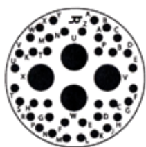
25-42 - 25-42* 38 #20, 4 #8 Coax I, Coax
