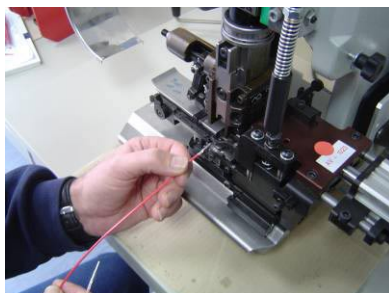
The picture shows crimping process with Mini-applicator
