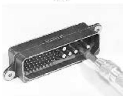
Extracting Coaxial & #12 Contacts
