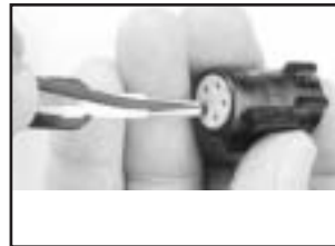
1. Open the CET - SLE Extraction tool and place it over the insulation of the wire.
