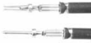
8. Note that there are no unterminated wire strands, and that some strand ends can be seen at the forward edge of the crimp. Also note the insulation is gripped by the smaller secondary crimp. Distortion is at a minimum, both axially and laterally - no sharp edges.
