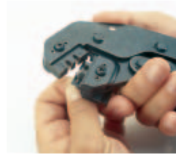
3. When correctly positioned the contact should be located beyond flush with the edge of the CCT - SLE / SLC and positioned in the concave polished split level crimp.
