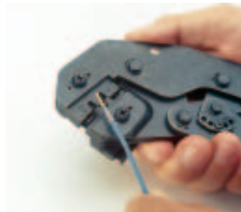
7. The result will be a perfect termination.
