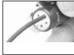
3. Continue the forward movement until an audible snap can be felt and heard. Slight pull in the opposite direction will confirm complete insertion.
