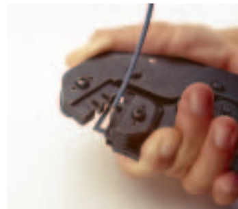
5. Insert the pre-stripped wire into the crimp area of the contact and completely cycle the tool.
