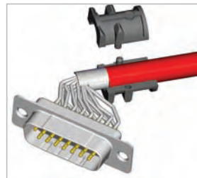
Attach the strain relief around the cable
