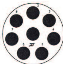
Series III Series II Series I No. of Contacts Service Ratings 25-8 - 25-8* 8 #8 Twinax Twinax I
