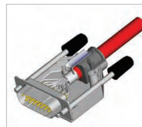
Mount connector and cable into the backshell
