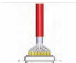
Strip cable 18mm and shape cable to two pigtails
