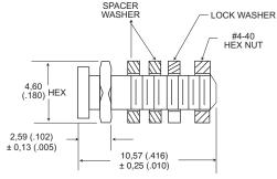
NOTE: When rear-mounting connector to a 1/16" panel, delete the second spacer washer.
