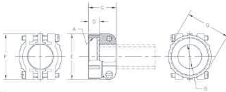
"A" Style Clamp With Bushing
