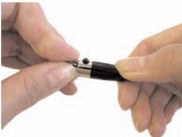
Rotate cap clockwise to thread onto connector housing to complete assembly. Perform a light pull test and visually inspect the finished assembly.
