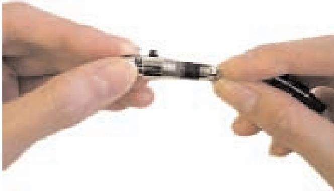
Insert complete sub-assembly into front barrel of connector. Please take extra precaution to orientate the barrel and sub-assembly during insertion. Keying feature has been added to ensure both components are positioned properly during this step.
