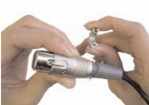
Finally, screw clamp onto the shell assembly to lock cable into position. Please take extra precaution to orientate clamp into its proper position. The inside chamfer with the largest diameter must butt against the shell assembly. Perform a light pull test and visually inspect finished assembly.
