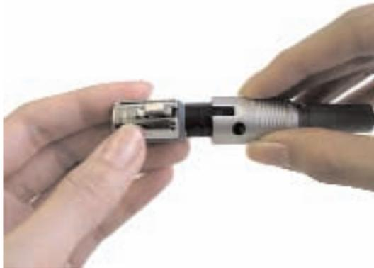
Supporting the insert assembly in one hand, slide the insulator tube and shell assembly into position, as shown.
