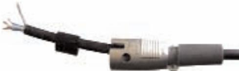
Slide shell assembly and insulator tube onto cable.
