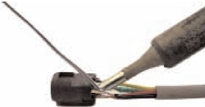
Preparing Insert Assembly; Solder individual center conductors to each contact. Visually inspect solder joints before proceeding.
