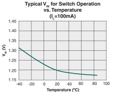
Typical Turn-On vs. Temperature (I,=100mA)
