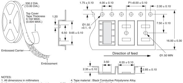
2. 10 sprocket hole pitch cumulative tolerance  $\pm$  0.20. 3. Carrier camber is within 1mm in 250mm.
