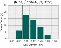
Typical I<sub>F</sub> for Switch Dropout
