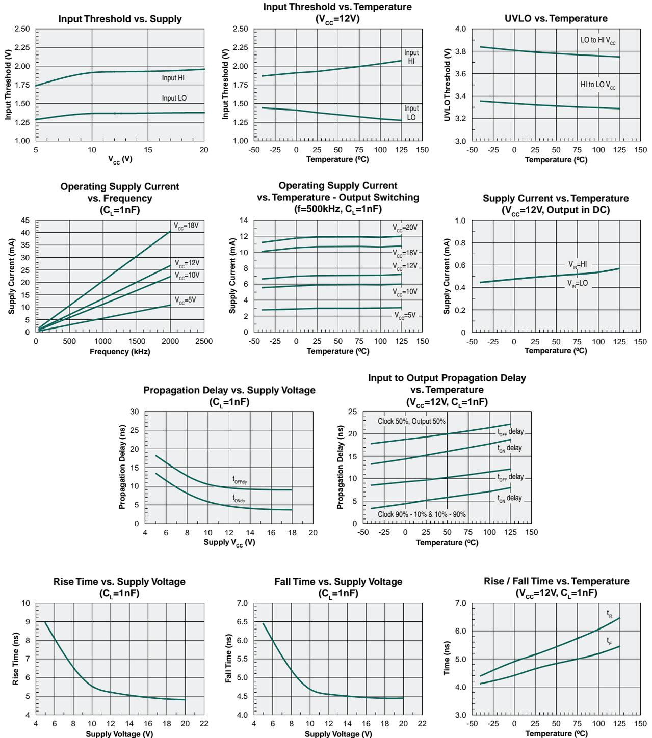
\*Unless otherwise noted, data presented in these graphs is typical of device operation at 25 $^{\circ}C$ .
