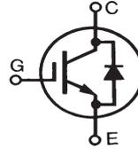
$$\begin{aligned} V_{CES} &= 1700 \text{ V} \\ I_{C25} &= 26 \text{ A} \\ V_{CE(sat)} &= 5.2 \text{ V} \\ t_{fi(typ)} &= 50 \text{ ns} \end{aligned}$$
