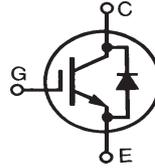
$$\begin{aligned} V_{CES} &= 1700 \text{ V} \\ I_{C25} &= 38 \text{ A} \\ V_{CE(sat)} &= 3.5 \text{ V} \\ t_{fi(typ)} &= 250 \text{ ns} \end{aligned}$$
