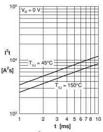
Fig. 3 I<sup>2</sup>t versus time per diode
