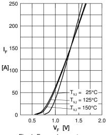
Fig. 1 Forward current versus voltage drop per diode
