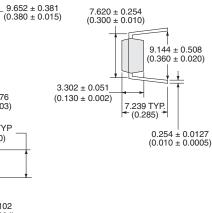
PCB Hole Pattern  $\begin{array}{c} 8-0.800 \text{ DIA.} \\ (8-0.031 \text{ DIA.}) \\ \hline \\ 6.350 \pm 0.127 \\ (0.250 \pm 0.005) \\ \hline \\ 7.620 \pm 0.127 \\ (0.300 \pm 0.005) \\ \hline \\ 7.620 \pm 0.127 \\ (0.300 \pm 0.005) \\ \hline \\ 7.620 \pm 0.127 \\ (0.300 \pm 0.005) \\ \hline \end{array}$
