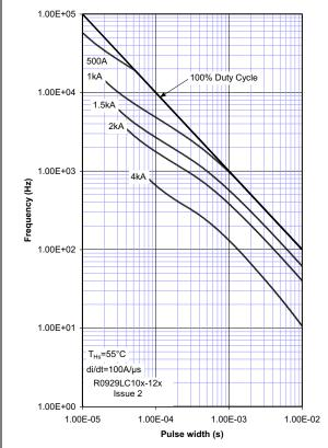
Figure 13 - Square wave frequency ratings
