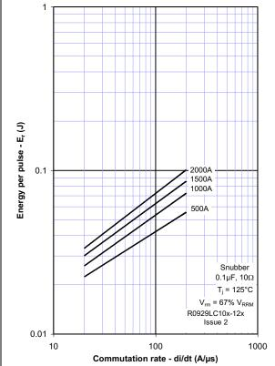
Figure 9 - Reverse recovery energy per pulse
