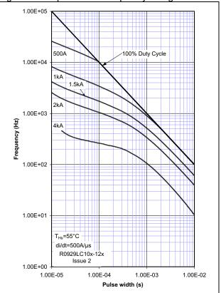
Figure 16 - Square wave frequency ratings
