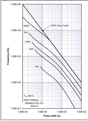
Figure 14 - Square wave frequency ratings
