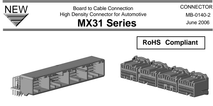
High density and non-water proof type of MX31 series is developed to meet the demands for compact and lighter connectors with multi pin counts, due to increase of computerized control in automotives. Pitch of signal terminal is 2.2mm, and the pitch of power terminal is 3.2mm. Compact and 4row type and the variation of the number of terminal is from 70pos. to 135pos. (pin header) This connector meets with automotive specs. and the application is for Automotive EUC (Engine, transmission, etc)
