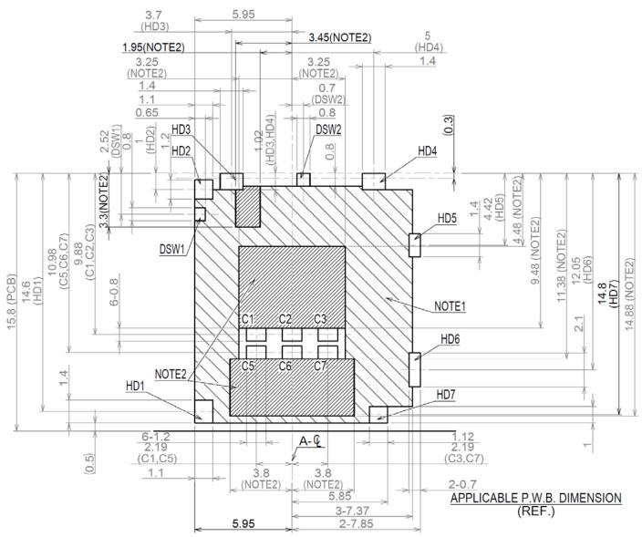
NOTE 1: ONLY GND PATTERN AND VIA HOLE IN ALLOWED IN THIS AREA. NOTE 2: NO PATTERN , NO VIA HOLE IN THIS AREA.
