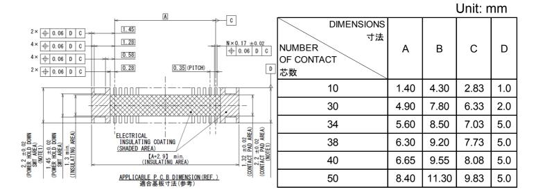
Note 1) Dimension 2.8  $\pm$  0.05 is recommended in case repair is needed.
