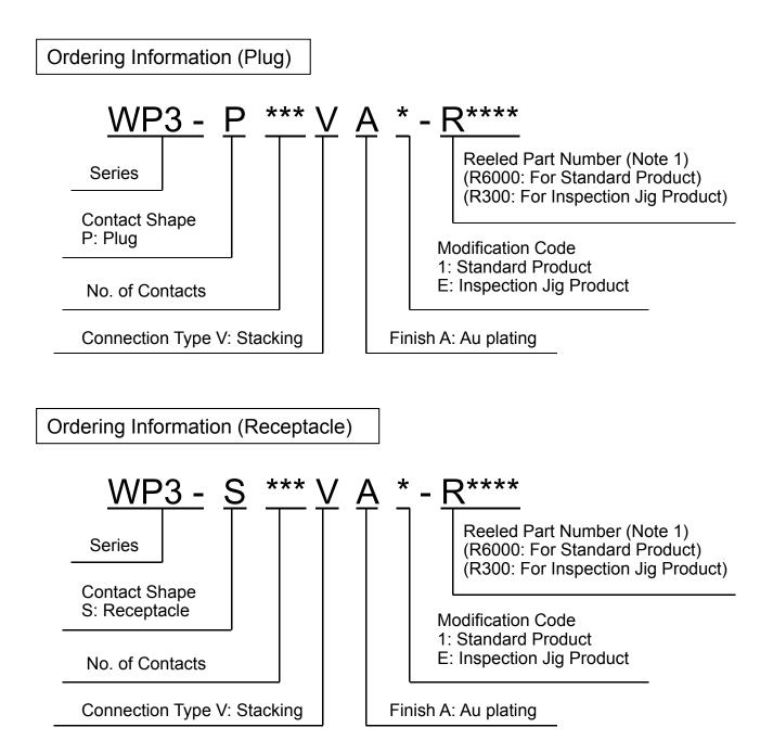
Note 1) An embossed tape reel contains 6,000 pieces of standard product, or 300 pieces of inspection jig product. Please contact us for details on embossed tape specifications.
