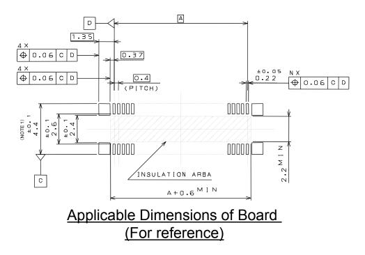
Note 1) Dimension  $3.8 \pm 0.05$  is recommended in case repair is not needed.
