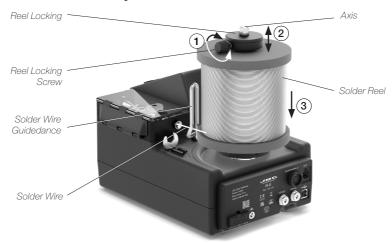
Open the reel locking screw (1) and remove the reel locking (2) from the axis.
