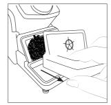
Remove the wiper by pulling it out.
