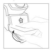
Lift the wiper at its front edge.
