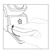
Lift the wiper at its front edge.
