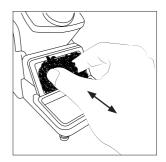
Replace the brass wool with a new one when it is worn out.
