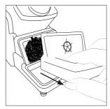
Remove the wiper by pulling it out.
