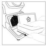
Remove the wiper by pulling it out.
