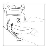
Lift the wiper at its front edge.
