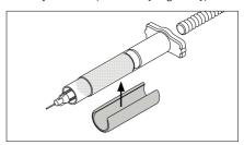
For 3cc syringes the adaptor is needed. Assemble the adapter by clipping onto the barrel.
