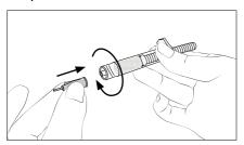
Thread the tip onto the syringe barrel.
