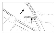
Open the DPM by lifting its upper part and the lever.
