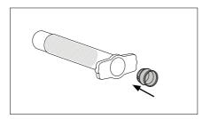
Take the barrel filled with solder paste and place the corresponding piston into the barrel.
