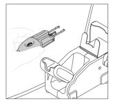
When the wire stripper is lifted from the stand, the cartridges will heat up according to the selected configuration.
