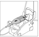
After longer periods of inactivity, the power is cut off and the cartridges cool down to room temperature.
