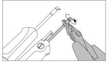
Align cartridges with JBC pliers.
