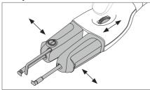
The wheel allows to adjuste the wire stripper arm position accordig to the wire diameter. Move the wheel backward for a wider and forward for a narrower position.
