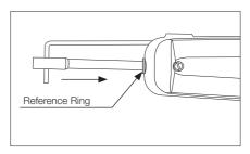
Insert the cartridge until the reference ring touch against the wire stripper. Take the ring as reference and check that both tips match.
