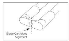
Align the tip edges and fix the cartridges in its working position.
