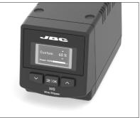
To work on a customized mode, press and then the buttons and to select the power level.
