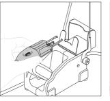
When the wire stripper is in the stand, the power falls after a specified time.
