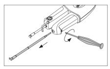
Loosen the screws and remove the cartridges.
