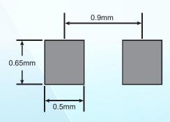
Print solder in thickness of 0.08mm to 0.10mm
