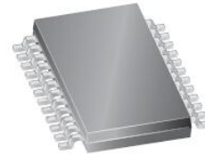
28 lead TSSOP with exposed thermal pad
