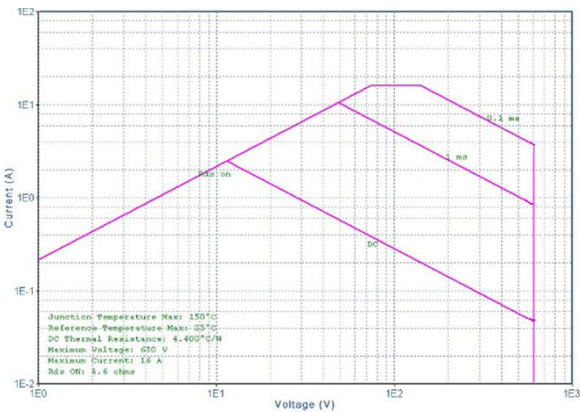
Maximum Safe Operating Area For JCS4N60FC(TO-220MF-K2)
