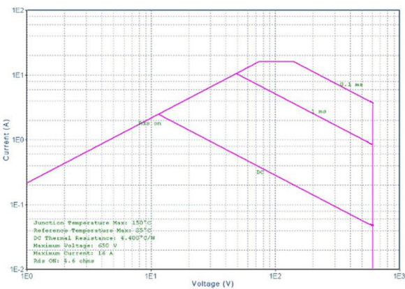
Maximum Safe Operating Area For JCS4N60FC(TO-220MF-K2)
