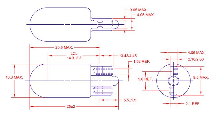
\*TO BE MEASURED ON LONGEST SIDE ONLY WITH THE WIRE IN INTIMATE CONTACT WITH THE BOTTOM OF THE GLASS WEDGE.
