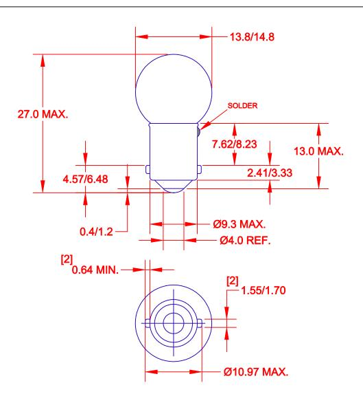
JKL LAMPVOLTAGEAMPERAGEWATTAGELUMENSLIFE HOURSFILAMENTOP21046.02.012.00100100C6U (FC6U)
