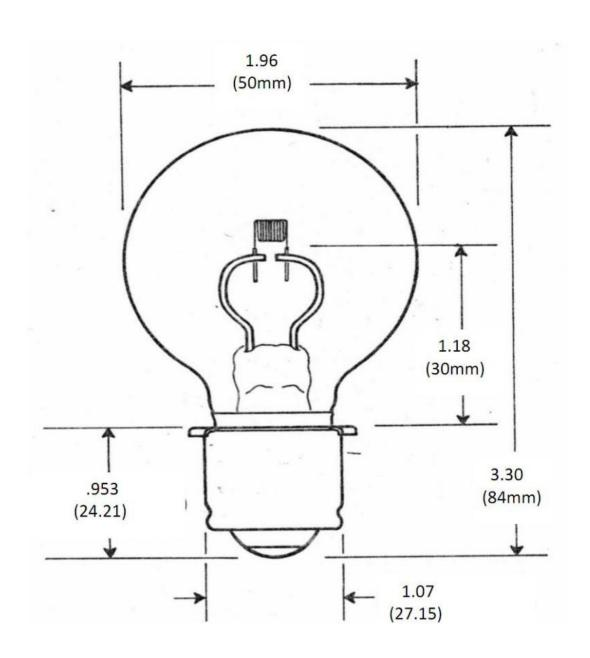
VOLTS AMPS WATTS LUMENS LIFE HOURS FILAMENT 12 8.3 100 1900 100 FC-6U
